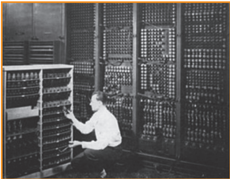
Fig. 1. ENIAC. The first multi-purpose fully electronic computer designed for calculations, based on vacuum tubes
