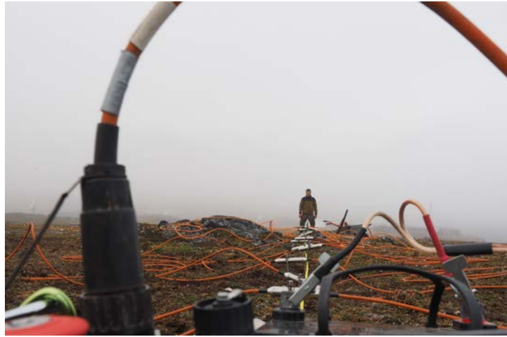
Geophysical measurements by electrical resistivity tomography are used to identify the features of permafrost and its active layer.
